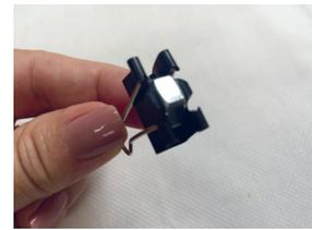
ENCAIXE O CLIPE NO EIXO DO MOTOR. PASSE COLA QUENTE.
